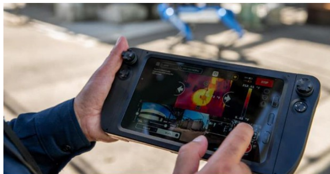
Exhibit 124: An operator uses Spot's CAM+IR capabilities to take visual and thermal images of equipment and gauges, which Chevron processes through its own computer vision program to detect anomalies
